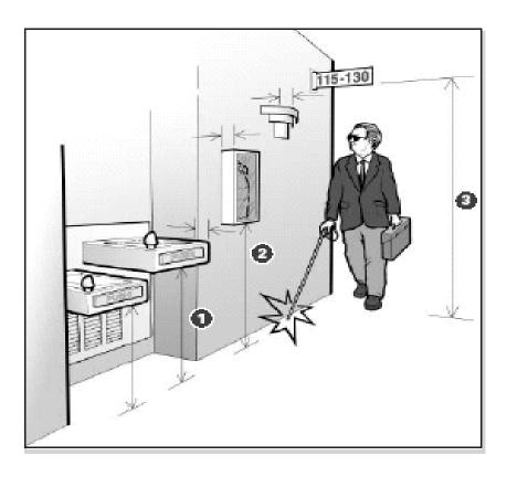
By placing a large planter under the wall mounted object as a detectable warning, this man could avoid an accident.
